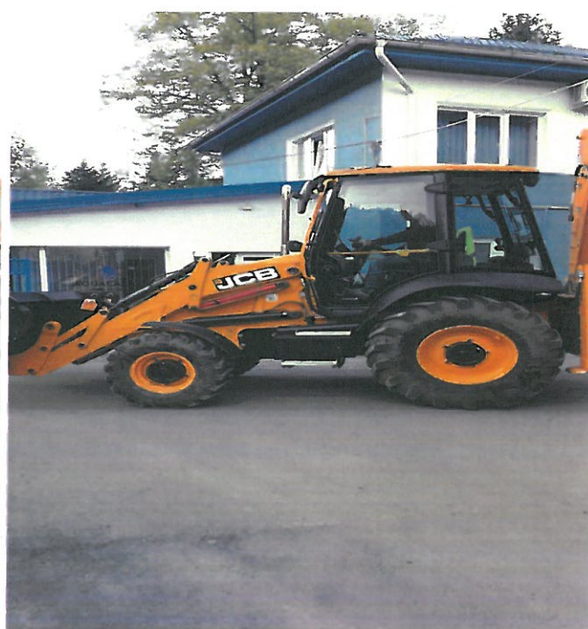
Poza 10. Buldoexcavator model JCB 3CX
